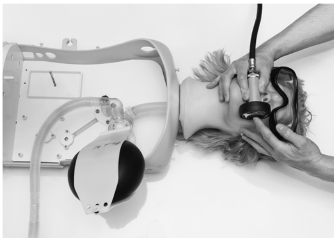
Figure 2 Test setting for the assessment of tidal volumes. The trachea-like hose of the manikin is connected to a non-re-breathable valve. The expiration branch is connected to the Primus ventilator to detect the expiratory tidal volumes of the test lung. The two-handed technique is used to operate the Poseidon Cyklon 5000 regulator. During ventilation with the Cyklon 5000, the test lung is overinflated.
