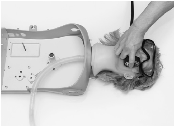
Figure 1 Test setting for the assessment of peak pressures. The hose attached to the upper airways of the manikin is directly connected to the Primus ventilator for pressure measurement. The one-handed technique is used to operate the SCUBA regulator.
